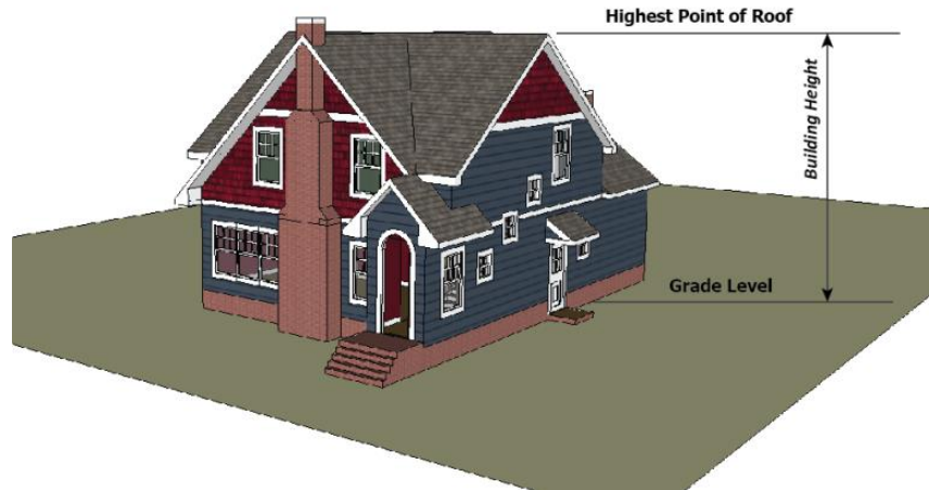
Figure 5.05-J: Measurement of building or structure height
